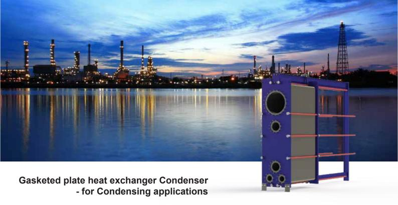
Baode Cond GPHE is a plate surface condenser designed for condensation under vacuum. Baode Condenser GPHE is based on semi-welded technology. Vapour condenes in the welded channel while the cooling medium passes through the gasketed channel. In addition to stainless steel, the plates are also available in titanium, which makes it possible to use seawater as a cooling medium.
